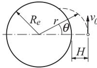
A spacecraft is launched at the altitude  $H = 772$  km above sea level with the speed  $v_0 = 6700$  m/s in the direction shown. The differential equations describing the motion of the spacecraft are
