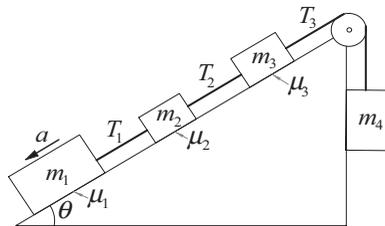
The four blocks of different masses  $m_i$  are connected by ropes of negligible mass. Three of the blocks lie on a inclined plane, the coefficients of friction between
