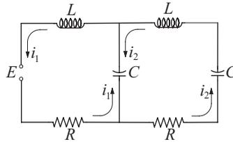
The constant voltage source of the circuit shown is turned on at  $t = 0$ , causing transient currents  $i_1$  and  $i_2$  in the two loops that last about 0.05 s. Plot these currents from  $t = 0$  to 0.05 s, using the following data:  $E = 9$  V,  $R = 0.25$   $\Omega$ ,  $L = 1.2 \times 10^{-3}$  H, and  $C = 5 \times 10^{-3}$  F. Kirchoff's equations for the two loops are
