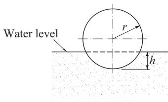
The equilibrium position of the floating cylinder is  $h = r$ . If the cylinder is displaced to the position  $h = 1.5r$  and released, the differential equation describing its motion is
