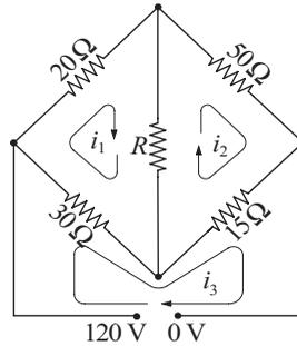
The electrical network shown can be viewed as consisting of three loops. Applying Kirchoff's law ( $\sum$  voltage drops =  $\sum$  voltage sources) to each loop yields the following equations for the loop currents  $i_1$ ,  $i_2$  and  $i_3$ :
