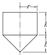
The cylindrical container has a conical bottom and an open top. If the volume  $V$  of the container is to be  $1.0 \text{ m}^3$ , find the dimensions  $r$ ,  $h$ , and  $b$  that minimize the surface area  $S$ . Note that
