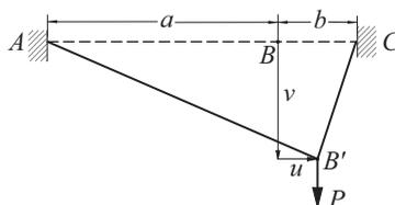
The elastic cord  $ABC$  has an extensional stiffness  $k$ . When the vertical force  $P$  is applied at  $B$ , the cord deforms to the shape  $AB'C$ . The potential energy of the system in the deformed position is
