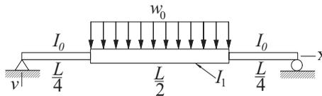
The simply supported beam consists of three segments with the moments of inertia  $I_0$  and  $I_1$  as shown. A uniformly distributed load of intensity  $w_0$  acts over the middle segment. Modeling only the *left half* of the beam, the differential equation
