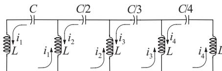
Determine the circular frequencies of oscillation for the circuit shown, given these Kirchoff equations:
