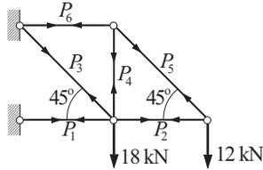
In the *force formulation* of a truss, the unknowns are the member forces  $P_i$ . For the statically determinate truss shown, force formulation is obtained by writing down the equilibrium equations of the joints
