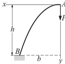
A uniform beam forms the semi-parabolic cantilever arch  $AB$ . The vertical displacement of  $A$  due to the force  $P$  can be shown to be
