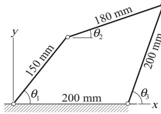
The three angles of the four-bar linkage are related by
