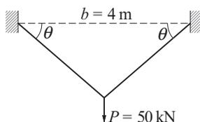
Each member of the truss has a cross-sectional area  $A$ . Find  $A$  and the angle  $\theta$  that minimize the volume
