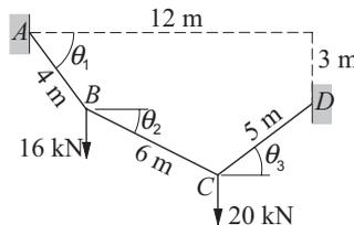
The 15-m cable is suspended from  $A$  and  $D$  and carries concentrated loads at  $B$  and  $C$ . The vertical equilibrium equations of joints  $B$  and  $C$  are
