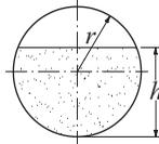
The cylindrical oil tank of radius  $r$  and length  $L$  is filled to depth  $h$ . The resulting volume of oil in the tank is
