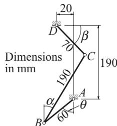
Geometric analysis of the linkage shown resulted in the following table relating the angles  $\theta$  and  $\beta$ :
