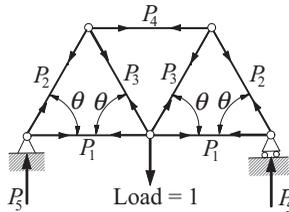
The force formulation of the symmetric truss shown results in the joint equilibrium equations
