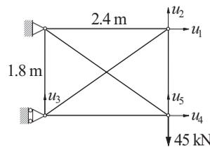
The displacement formulation for a plane truss is similar to that of a mass-spring system. The differences are (1) the stiffnesses of the members are  $k_i = (EA/L)_i$ , where  $E$  is the modulus of elasticity,  $A$  represents the cross-sectional area, and  $L$  is the length of the member; and (2) there are two components of displacement at each joint. For the statically indeterminate truss shown, the displacement formulation yields the symmetric equations  $\mathbf{Ku} = \mathbf{p}$ , where
