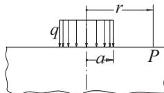
The figure shows an elastic half-space that carries uniform loading of intensity  $q$  over a circular area of radius  $a$ . The vertical displacement of the surface
