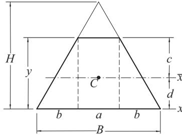
where  $I_{\bar{x}}$  is the second moment of the cross-sectional area about the axis that passes through the centroid  $C$  of the cross section. By optimizing the section modulus, we minimize the maximum bending stress  $\sigma_{\max} = M/S$  in the beam,  $M$  being the bending moment.
