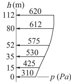
The pressure of wind was measured at various heights on a vertical wall, as shown on the diagram. Find the height of the pressure center, which is defined as
