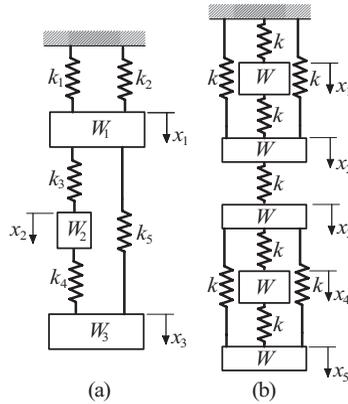
13. ■ The equilibrium equations of the mass-spring system in Fig. (b) are
