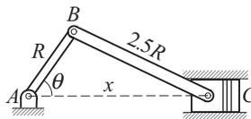
The crank  $AB$  of length  $R = 90$  mm is rotating at a constant angular speed of  $d\theta/dt = 5000$  rev/min. The position of the piston  $C$  can be shown to vary with
