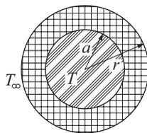
A wire carrying an electric current is surrounded by rubber insulation of outer radius  $r$ . The resistance of the wire generates heat, which is conducted through the insulation and convected into the surrounding air. The temperature of the wire can be shown to be
