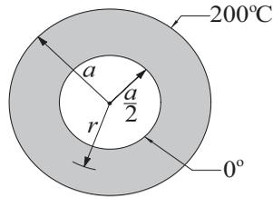
The thick cylinder conveys a fluid with a temperature of  $0^\circ\text{C}$ . At the same time the cylinder is immersed in a bath that is kept at  $200^\circ\text{C}$ . The differential equation and the boundary conditions that govern steady-state heat conduction in the cylinder are
