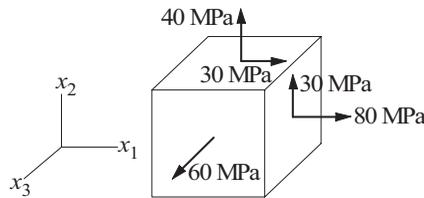
The stress matrix (tensor) corresponding to the state of stress shown is
