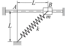
The sliding weight of mass  $m$  is attached to a spring of stiffness  $k$  that has an undeformed length  $L$ . When the mass is released from rest at  $B$ , the time it takes to reach  $A$  can be shown to be  $t = C\sqrt{m/k}$ , where
