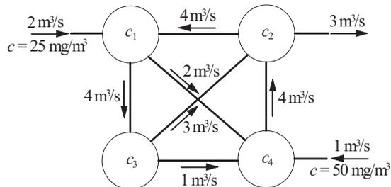
Four mixing tanks are connected by pipes. The fluid in the system is pumped through the pipes at the rates shown in the figure. The fluid entering the system contains a chemical of concentration  $c$  as indicated. Determine the concentration of the chemical in the four tanks, assuming a steady state.
