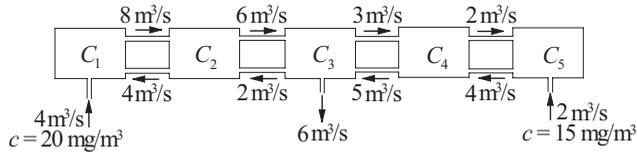
The diagram shows five mixing vessels connected by pipes. Water is pumped through the pipes at the steady rates shown on the diagram. The incoming water contains a chemical, the amount of which is specified by its concentration  $c$  ( $\text{mg}/\text{m}^3$ ). Applying the principle of conservation of mass
