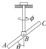
The bar  $ABC$  is attached to the vertical rod with a horizontal pin. The assembly is free to rotate about the axis of the rod. Neglecting friction, the equations of motion of the system are
