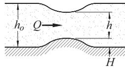
Bernoulli's equation for fluid flow in an open channel with a small bump is
